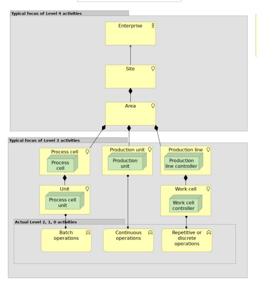
Based on ISA-95 Part 1 Figure 3, Page 19, Figure 4, page 23. This view applies the ArchiMate definition of location "A location is defined as a conceptual point or extent in space." to machinery as well, since machinery occupies space. All machinery is assumed also to have a processing capacity, i.e. a node that can run control applications, including ones that are embedded.
